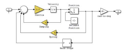
The Hard Stops block models the valve angular position limit of 15° to 90°.
