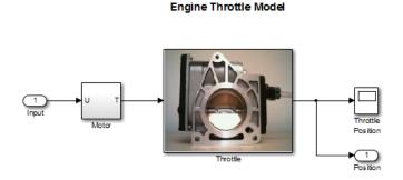
The throttle system controls the flow of air and fuel mixture to the engine cylinders. The throttle body contains a butterfly valve that opens when a driver presses the accelerator pedal. Opening this valve increases the amount of fuel mixture entering the cylinders, which increases the engine speed. A DC motor controls the opening angle of the butterfly
